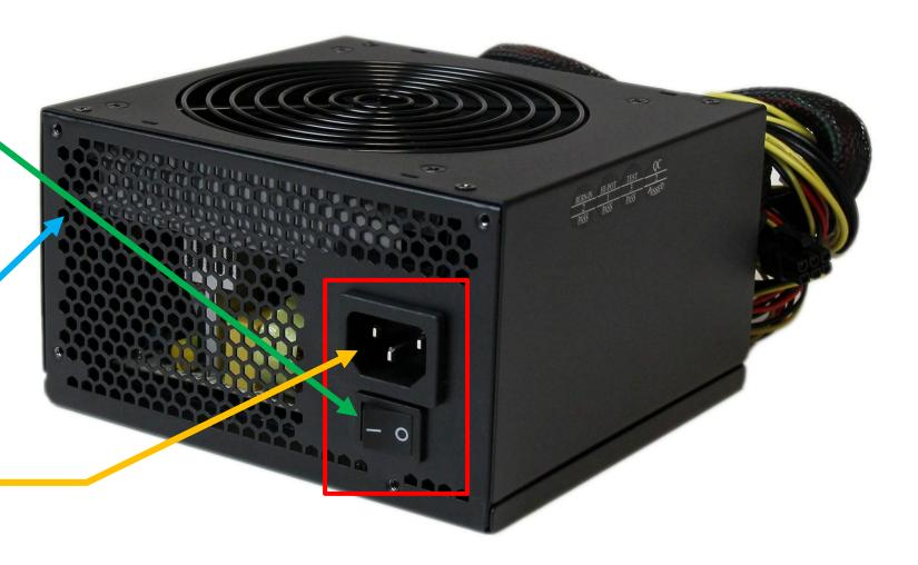
A main function of the PSU: convert the main AC to low voltage required to power a computer's components
