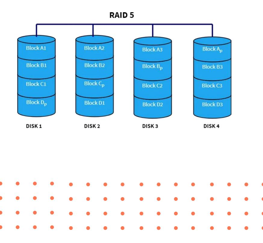
**Parity** – a calculated value that's used to mathematically rebuild data in case of a failure
